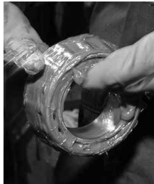
Fig. 23. Grease can easily be packed by hand.
